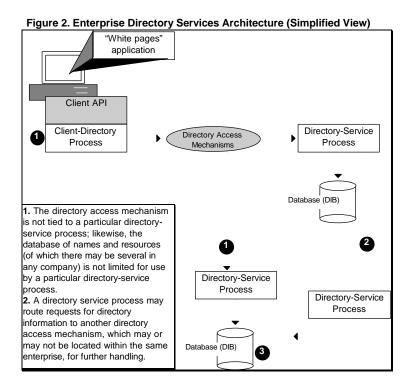
A **client-directory process** that enables an individual or another client application to make use of the information housed in the database. Applications on the desktop share a common client API.
