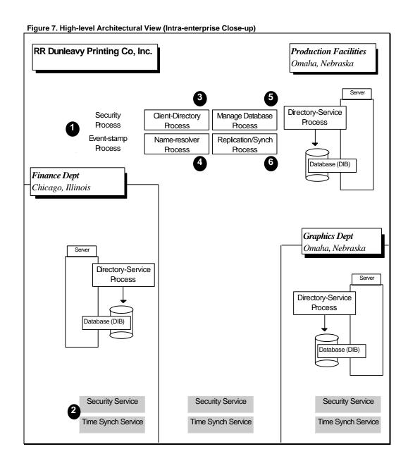
Before using any network resource, the identity and access-rights associated with the requesting person (or process) must be validated by a security process, with the event recorded in the log.
